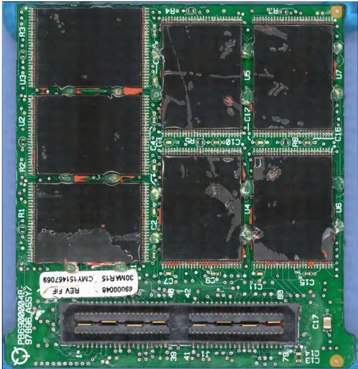
Figure 1.CVR memory module board,connector side.
