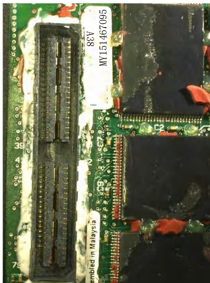
Figure 3. Detail of CVR memory module connector, as received.
